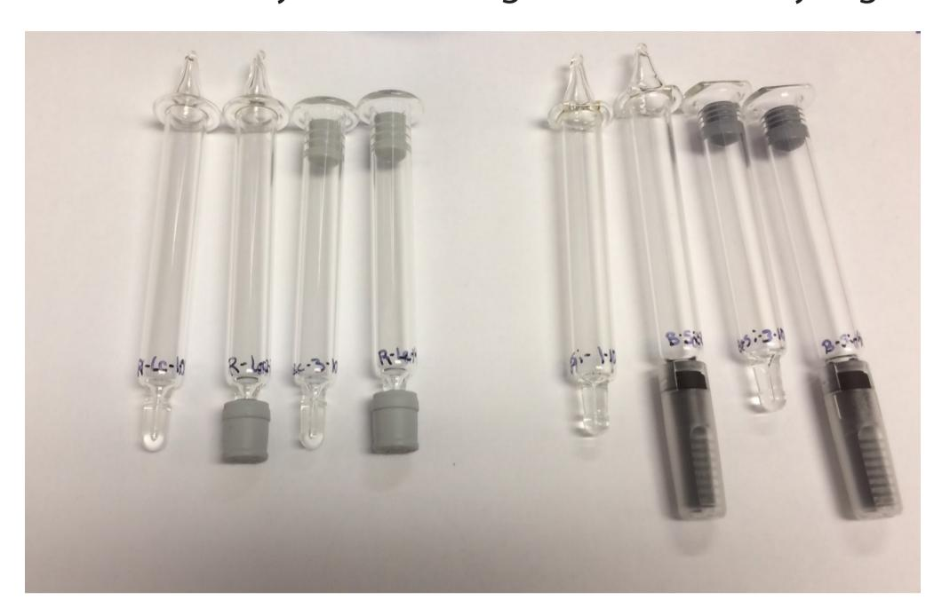
Figure 2. Sample syringes showing how various parts of the syringe can be isolated for study of oxygen ingress. Two types of syringes were studied (staked needle and Luer tip) as well as negative controls (completely flame sealed) and positive controls (flame sealed with micron size laser drilled defects)
