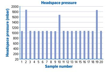
Data which identified three media vial samples that temporarily leaked while stored on dry ice. Cold dense carbon dioxide gas ingressed into the vials during cold storage and was trapped after the vials resealed when taken out of storage. This trapped gas resulted in depleted oxygen, and elevated carbon dioxide and pressure levels in the headspace of the vials that leaked.
