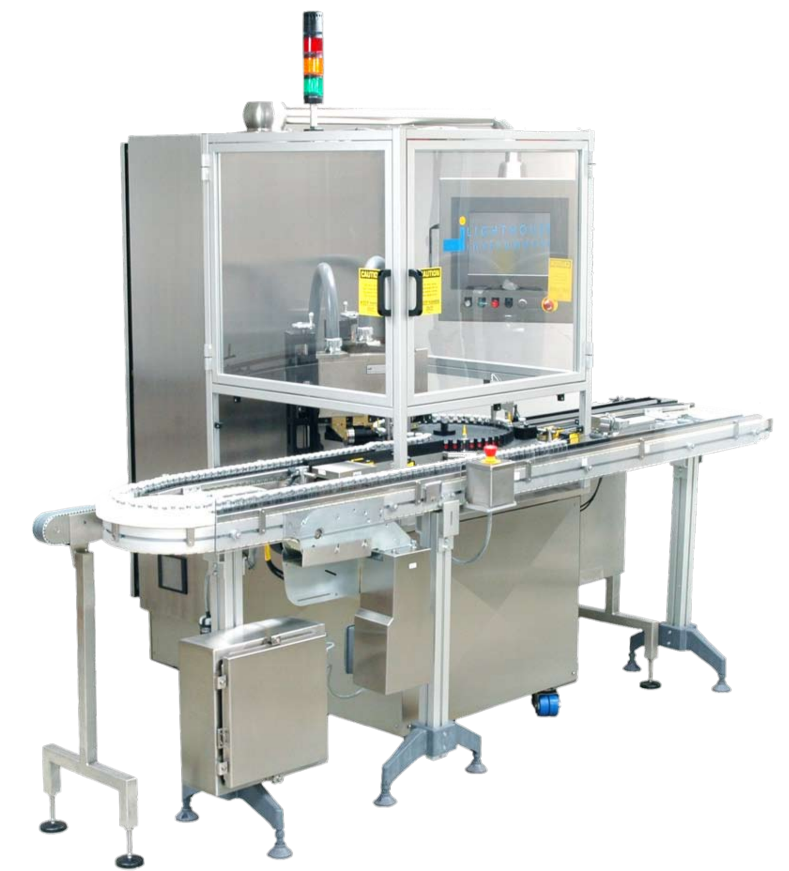
Automated headspace moisture/vacuum inspection machines have been implemented and qualified in the industry over the last five years for vacuum leak detection of freeze-dried vials at speeds up to 250 vials/min. Some of these machines are now also being validated for 100% moisture inspection.
